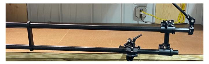
Attach the Forward facing sonar onto the 72" shaft. When transducer is in forward view, aline the transducer with the arrow indicator on top of the 72" pole. Use zip ties with Cobra cable clips to secure the transducer wires. Humminbird Live, you will not need the Cobra cable clips.
